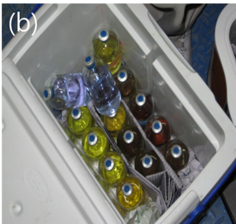
Fig. 1. Photographs of (a) groundwater sampling from the KURT (KAERI Underground Research Tunnel) and (b) several serum bottles containing nutrient media and KURT groundwater injected.
