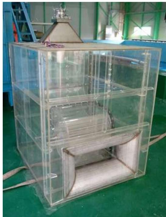
Fig. 6 Model of breakwater wave power generation system
