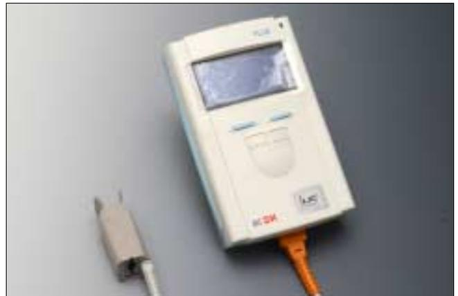
Fig. 4. MP110 pulse oximeter with probe.
