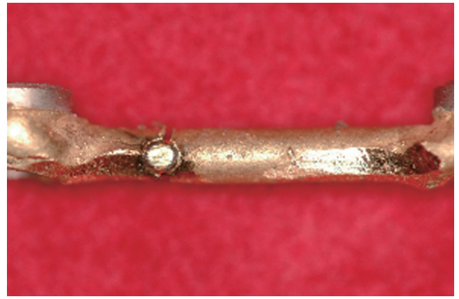
Fig. 3. Two-point laser welding for the specimens of group 3 (laser welding group) before additional soldering reinforcement. Two-point laser welding vertically directed to buccal and lingual side fused the opposing edges.
