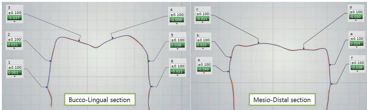
Fig. 4. 2D images converted from a 3D image using Convince software. The green boxes present the discrepancy at each registered point.
