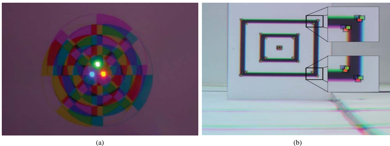
Fig. 7. (a) Overlapped RGB color images acquired by the proposed integral imaging system, (b) a sample overlapped RGB color image with color features on which the disparity is measured.
