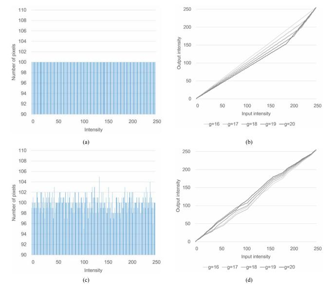
Fig. 1. Transformation functions for each level of the histogram grouping by GLG (a) Uniform histogram, (b) Transformation functions by the grouping of (a), (c) Histogram changed randomly, (d) Transformation functions by the grouping of (c).
