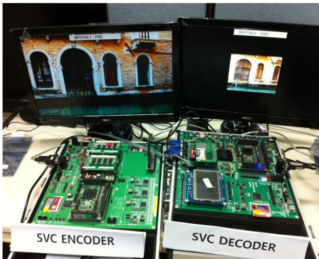
Fig. 6. Spatial SVC Encoder FPGA Verification.
