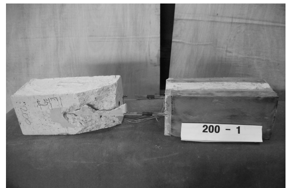
Fig. 4 Concrete failure from bond test
