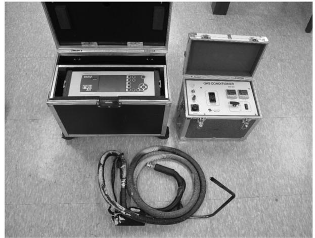
Fig. 1. Portable emission measuring system.
