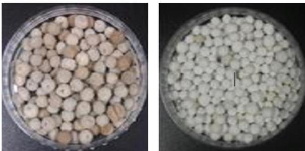
Fig. 3. Ball type filter for NOx(left) and SOx(right) reduction.
