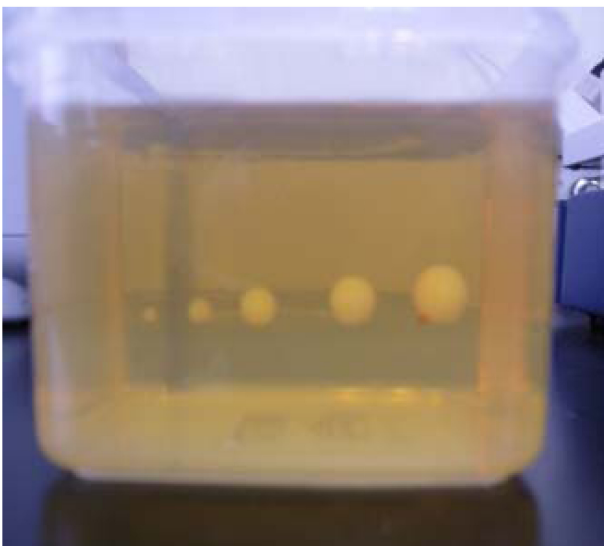
Fig 1. Artificial calculi phantom used for computed tomography.
