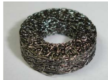
Fig. 1 Configuration of Pseudoelastic SMA MeshWasher[2]
