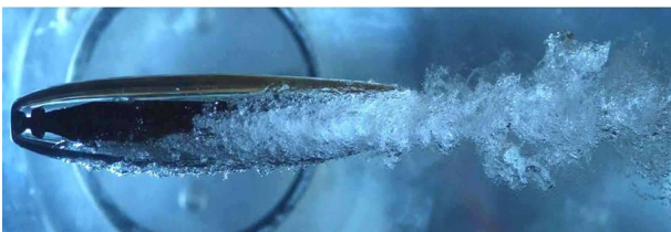
Fig. 9 Supercavitating underwater vehicle, picture taken from Wosnik, et al. (2003)
