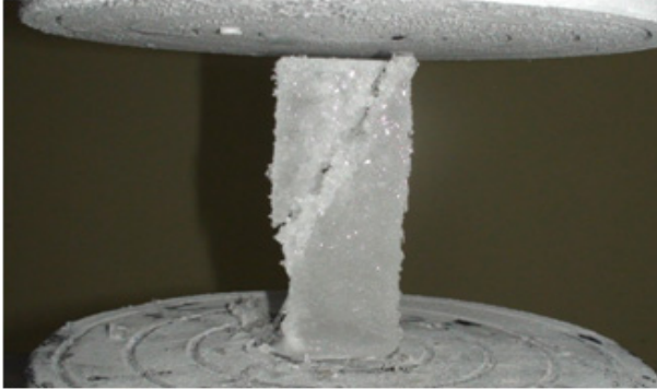
Fig. 5 Compressive strength test of model ice
