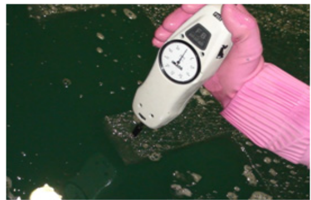
Fig. 4 Cantilever beam flexible strength test
