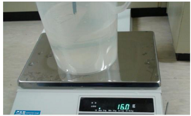
Fig. 7 Model ice density test
