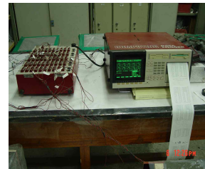
1) Measuring autogenous shrinkage by data logger
