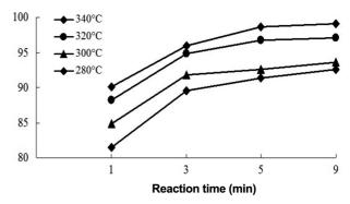
*Figure* **3.** Effect of temperature on WPO of oily wastewater. Conditions: residence time 1 to 9 min, HE 0.75, initial COD 18000 mg/L.
