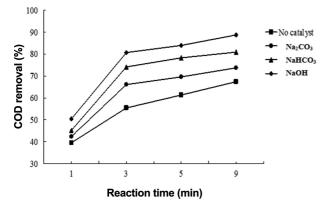
Figure 2. Effect of catalysts on COD removal.
