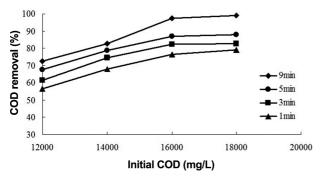
Figure 4. Effect of initial COD on WPO of oily wastewater.
