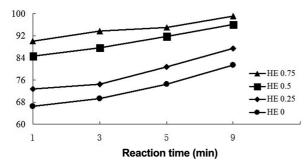
*Figure 5.* Effect of HE on WPO of oily wastewater. Conditions: temperature 340 °C, residence time 1 to 9 min, initial COD 18000 mg/L.
