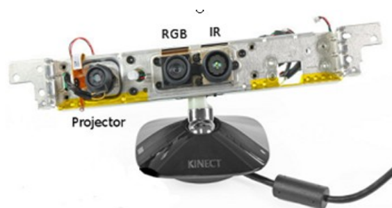
Fig.1. Kinect consists of Infrared (IR) projector, RGB camera and IR camera
