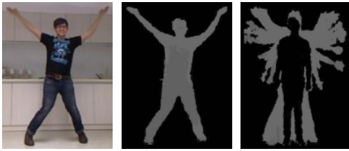
Fig. 5 From left to right: RGB Image, Depth Map and DMHI of jacking action
