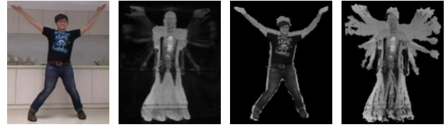
Fig. 4. from left to right columns: RGB Image, traditional MHI, RGB filtered by depth and RDMHI of jacking action respectively
