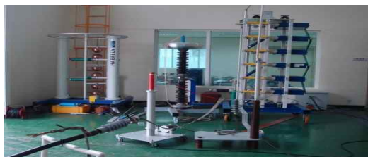
(a) Current impulse injection with ICG
