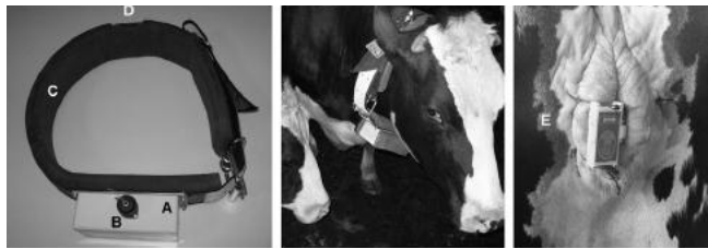
Fig. 11 A: Plastic box with a transmitter-receiver, B: Small USB connector, C: Polyethylene cushion, D: GPS/GSM antenna, E: Transceiver installed on external genitals (p. 125, Calcante, 2014)
