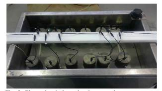
Fig. 2. Electrochemical accelerating corrosion test.
