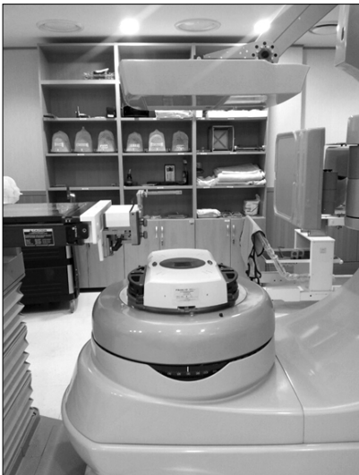
Fig. 9. The image of EPID setup for Winston Lutz Test at gantry 180° and Table 0°.
