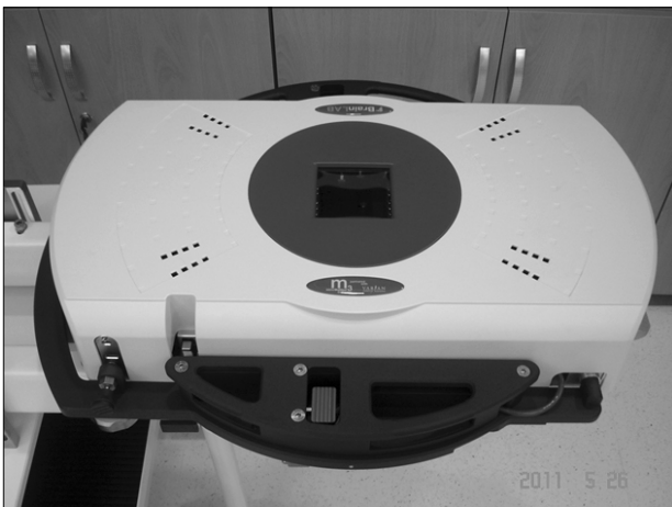
Fig. 2. Image of micro-multileaf collimator (m3, BrainLab).
