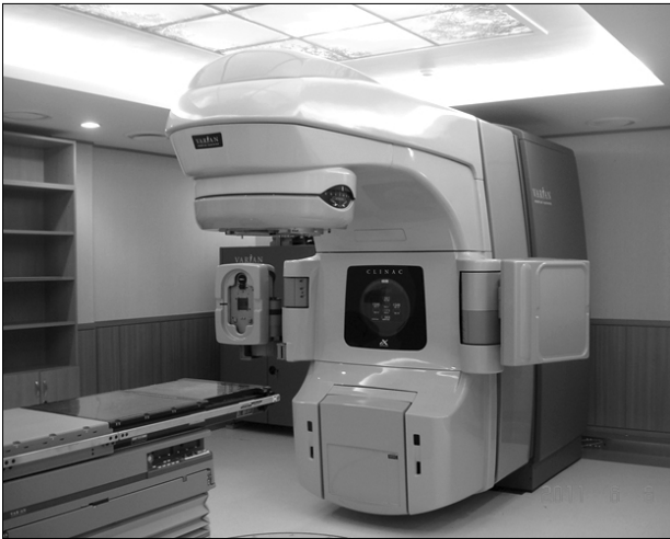
Fig. 1. Clinical linear accelerator (RapidArc Varian Co.).
