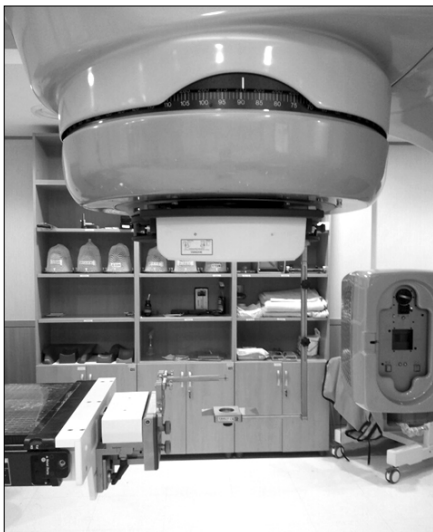
Fig. 6. The image of film setup for Winston Lutz Test at gantry 0° and Table 0°.
