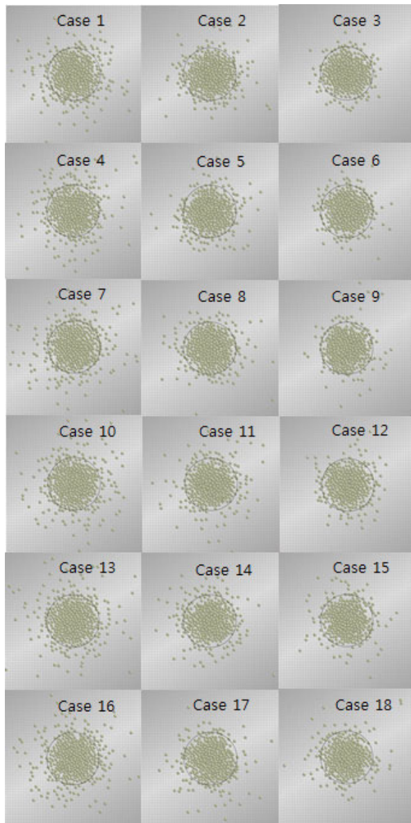
Fig. 16 Aggregate Slump Test Simulation for 19mm Aggregates in DEM
