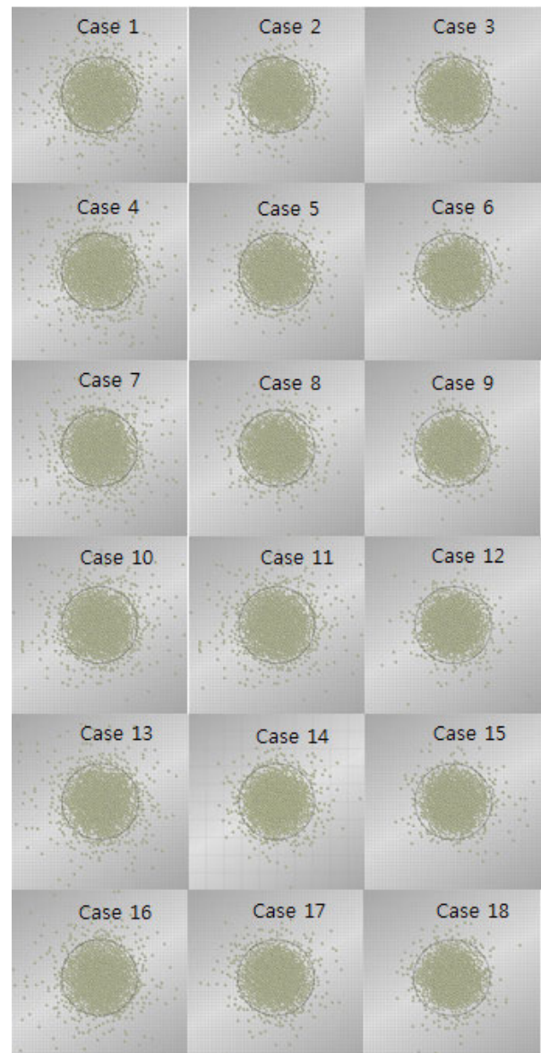
Fig. 17 Aggregate Slump Test Simulation for 13mm Aggregates in DEM
