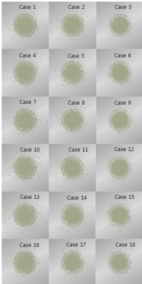
Fig. 18 Aggregate Slump Test Simulation for 10mm Aggregates in DEM
