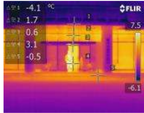
Fig. 6. Thermal imaging analysis of frontal entrance/exit
