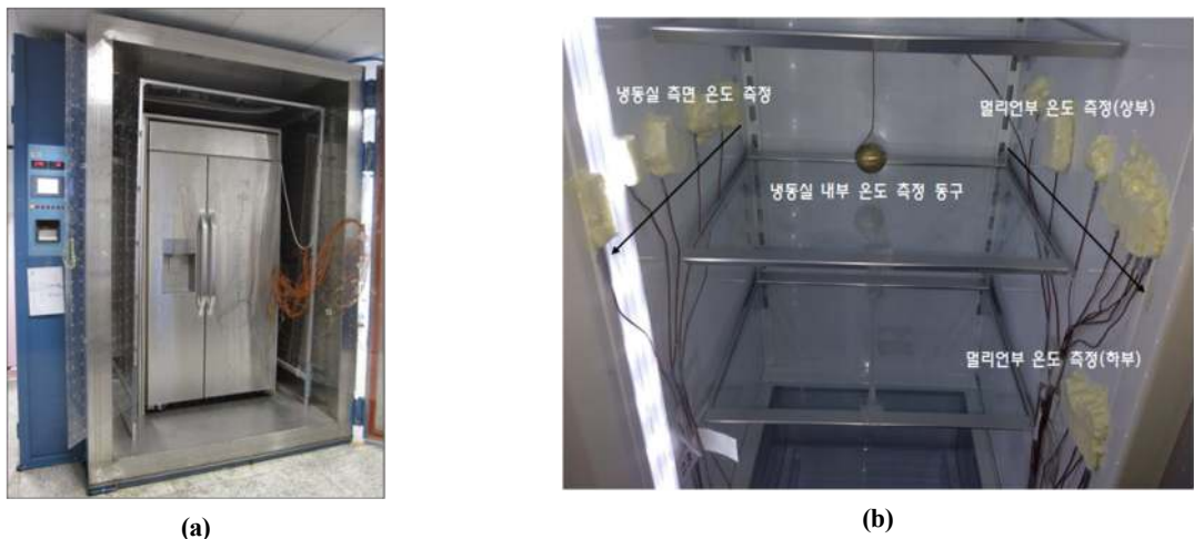
Fig. 1. Photograph of (a) test refrigerator in a constant temperature and constant humidity chamber and (b) thermocouple installation at the mullion side wall and freezer side wall.
