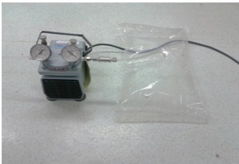
<Figure 2> Device for the Combustion Gas
