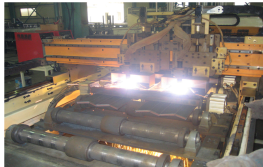
[Fig. 9] Cutting test of the flat-iron system in field
