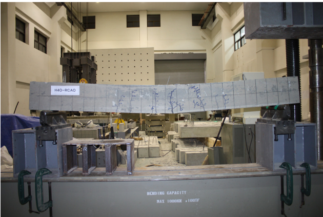
Photo 2 Crack pattern and failure mode of specimens
