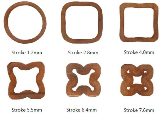
Fig. 7 The deformed specimen shapes under punch stroke of single round copper pipe
