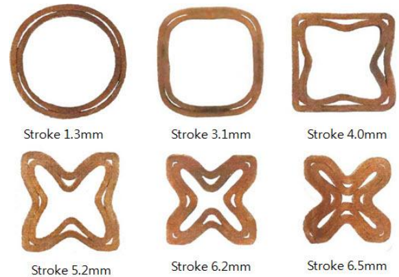
Fig. 8 The deformed specimen shapes under punch stroke of double round copper pipe
