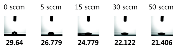
Figure 1. Contact angle images of the N-doped ethylcyclohexane plasma polymer thin films deposited at plasma power of 60 W and with changing the NH_3 flow rate from 0 to 50 sccm.
