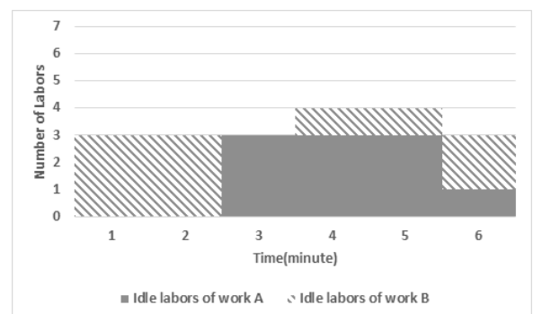
Fig. 8. Idle labors after application of multi-skilled laborers
