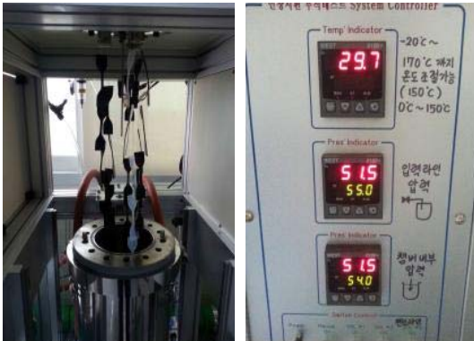
Fig. 5. Immersion test of the rubber specimens.
