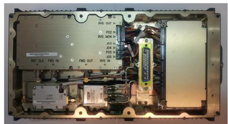
Fig. 4. Inner structure of mobile station RF module
