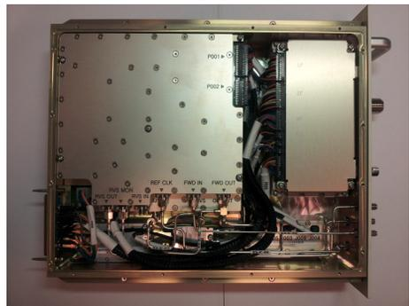
Fig. 3. Inner structure of base station RF module
