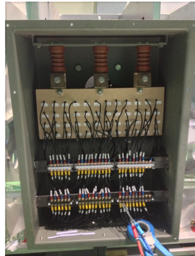
Fig. 8. Measurement of phase resistance and back-emf
