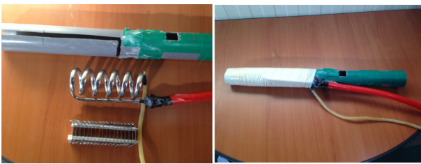
Fig. 2. Pipe with the pad and the cooling coil.
