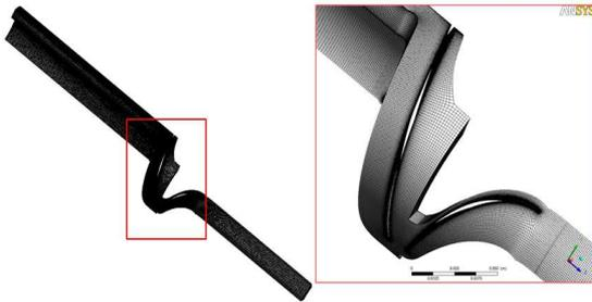
Fig. 8 Grid for the numerical analysis of base model impeller and diffuser
