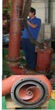
Fig. 10 Photo of pump performance test for verification
