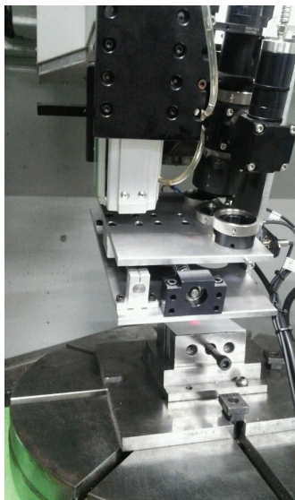
(b) The linear laser module
