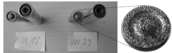
Fig. 5 Tools and electrodes after spark discharge
