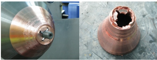
Fig. 13 Attachment of keys on mandrel (left) and failure during spinning process of nozzle throat part (right).
