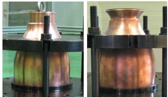
Fig. 18 Bulging test of spined nozzle throat inner wall, before bulging (left) and after bulging (right).
