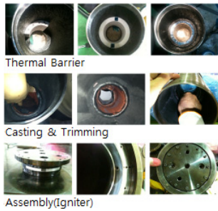
Fig. 6 Fabricating process of dual pulse motor.
