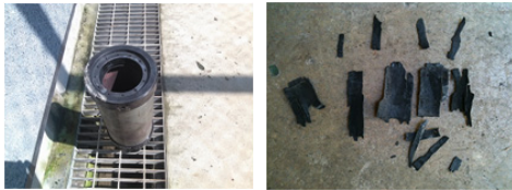
Fig. 11 Result of case and thermal barrier after 1st test for 2nd pulse motor.
