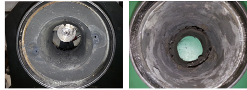
Fig. 13 Result of thermal barrier after 2nd/3rd test for 2nd pulse motor.
