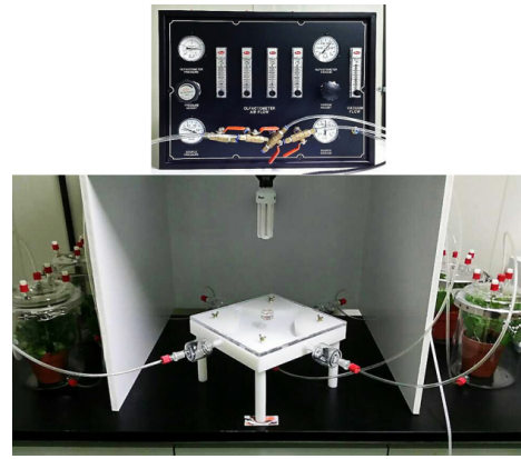
Fig. 1. Olfactometer system: a four-choice acrylic olfactometer connected to an air delivery system.
