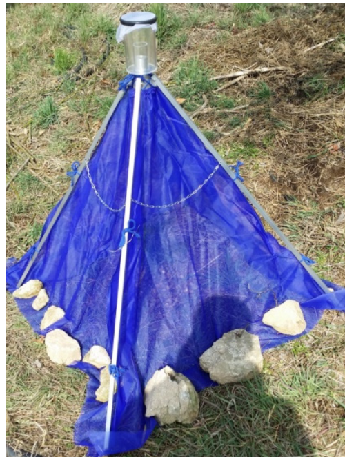
Fig. 1. Cone trap for adult wasp emergence monitoring in a Japanese apricot orchard.
