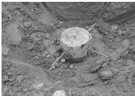
(a) Insert of four rebars in a wood pile
