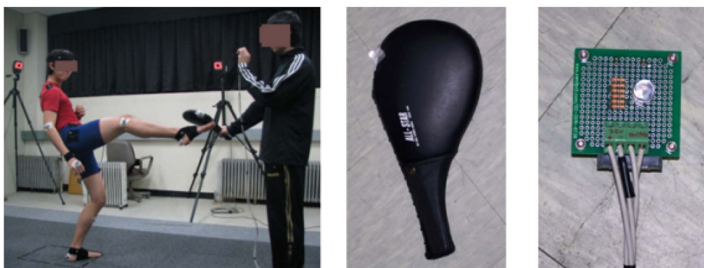
Figure 2. Experimental set-up, target with a marker, and LED for trigger signal to a kicker
