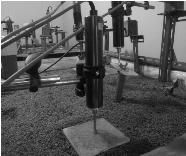
(a) Measurement of heave amount
