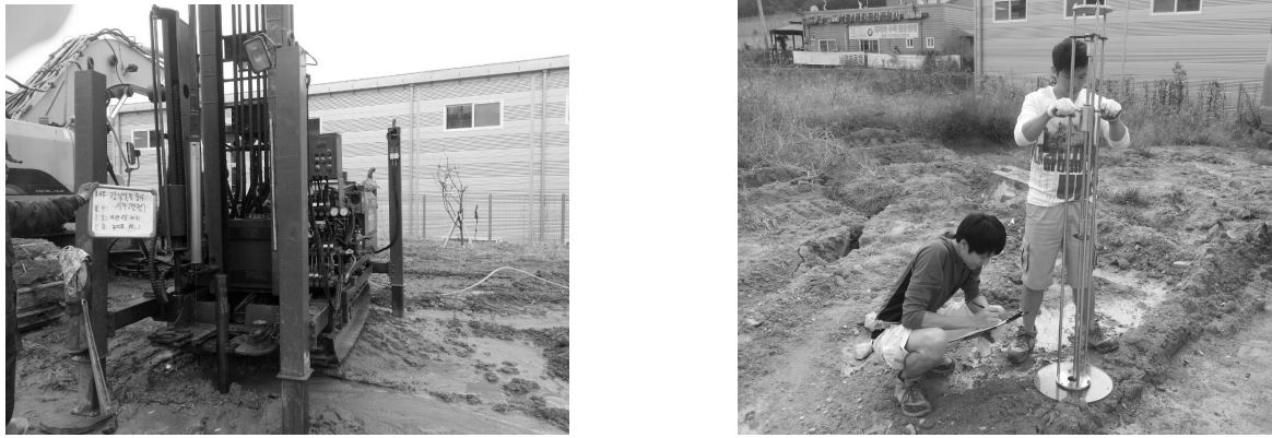
Fig. 12. Boring investigation and advanced cone penetration test (in Paju)
