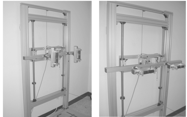
[Figure 1] Illustration of vertical handle type(left) and horizontal handle type(right)
