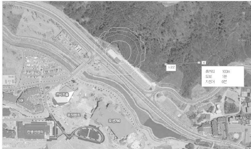
[Figure 6] Individual risk contour of A facility (with water spray)
