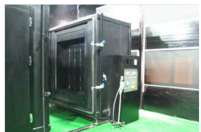
(c) Metering box
