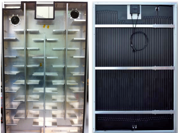
(a) Air duct (b) Water tube Fig. 2 PVT thermal collector.
